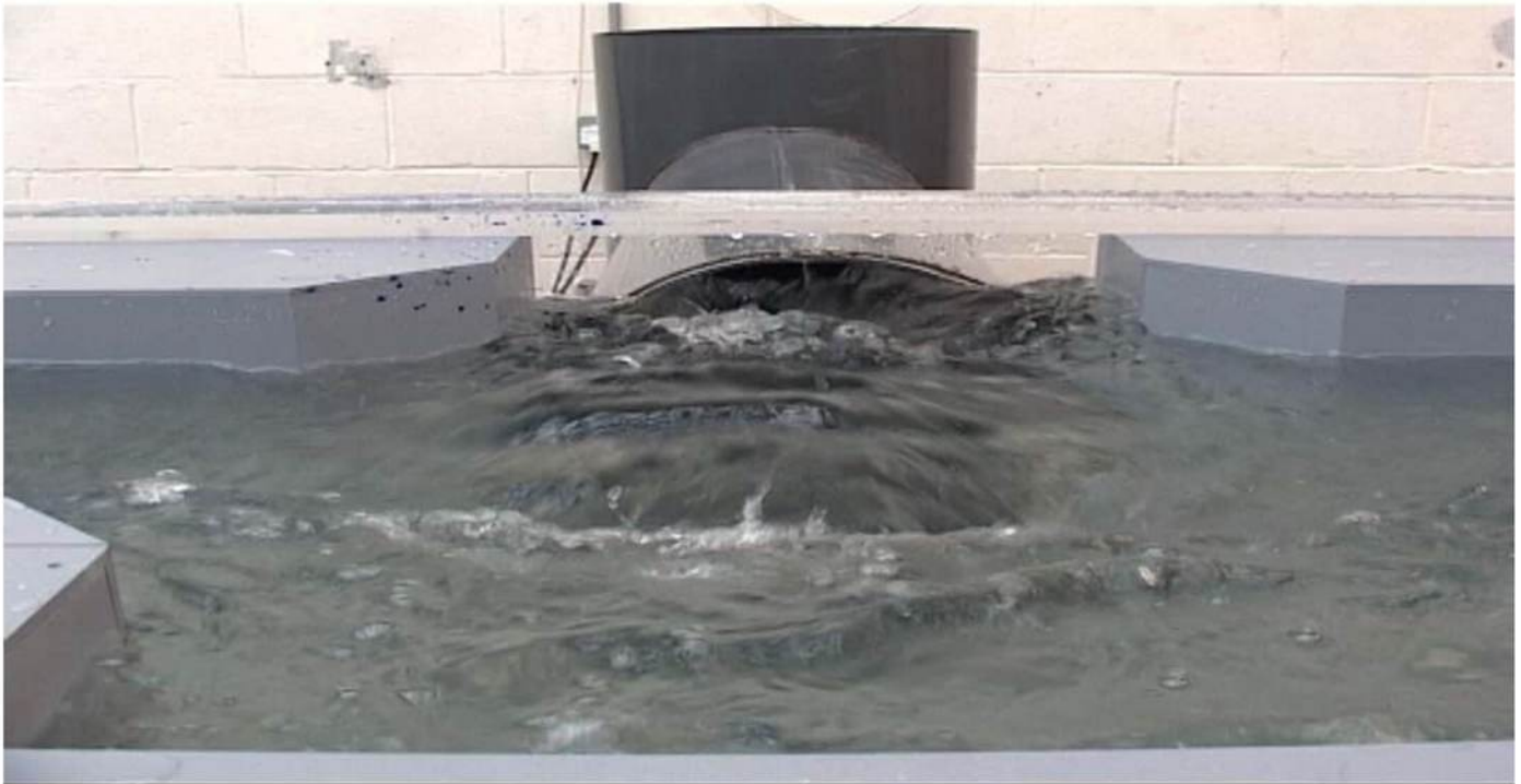
Fore bay (12 m 3 /s) Ultimate Flow Conditions
